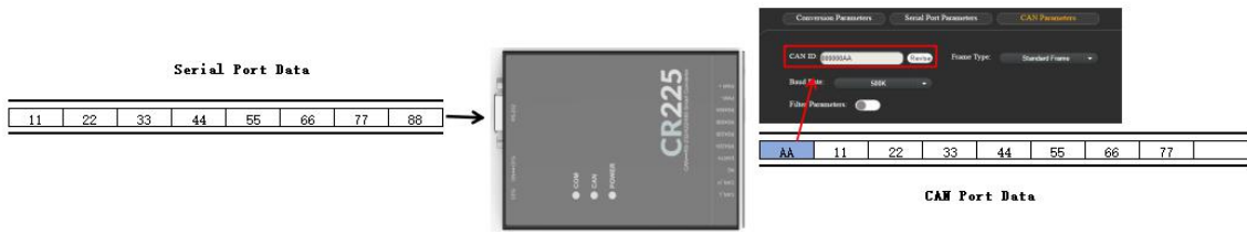
Figure 2 Serial frame length is less than or equal to 8 bytes
