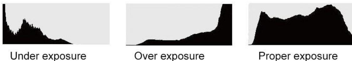
The video is likely being clipped if the information bunches to a hard edge at 0% or above 100% along the horizontal scale. Video clipping is undesirable when shooting, as detail in the blacks and whites must be preserved if the user subsequently wants to perform color correction in a controlled environment. When shooting, try to maintain the exposure so
