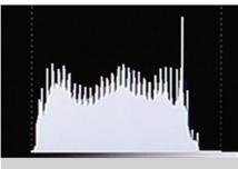
A display that indicates how many pixels of the screen are at a particular brightness level.
