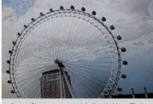
Areas of image over a certain threshold are filled with striped pattern to dramatically highlight areas where too much light is falling on image sensor.
