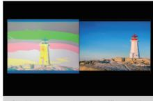
Special colors are used to indicate different levels of brightness in the image. Support ARRI, RED
