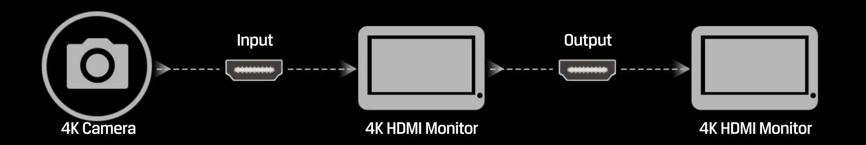
Equipped with HDMI 2.0 input/output interfaces, it can support up to 4096×2160 60p
