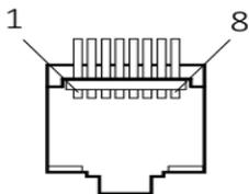
The GPI function is activated when the GPI pin is connected with the ground, and closed when it is disconnected from the ground. Connect to GPI to control the monitor remotely.
